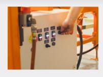
Operator-controlled adjustable feed speed sets the rate of the conveyor for adequate curing time
