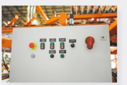
In addition, the control panel features the conveyor feed speed, lamp testing, and an emergency stop for safety. A self-contained electrical panel protects important wiring from the production environment.
