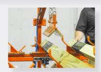
Pneumatic press applies even compression to square posts for a bubble-free sleeve application
